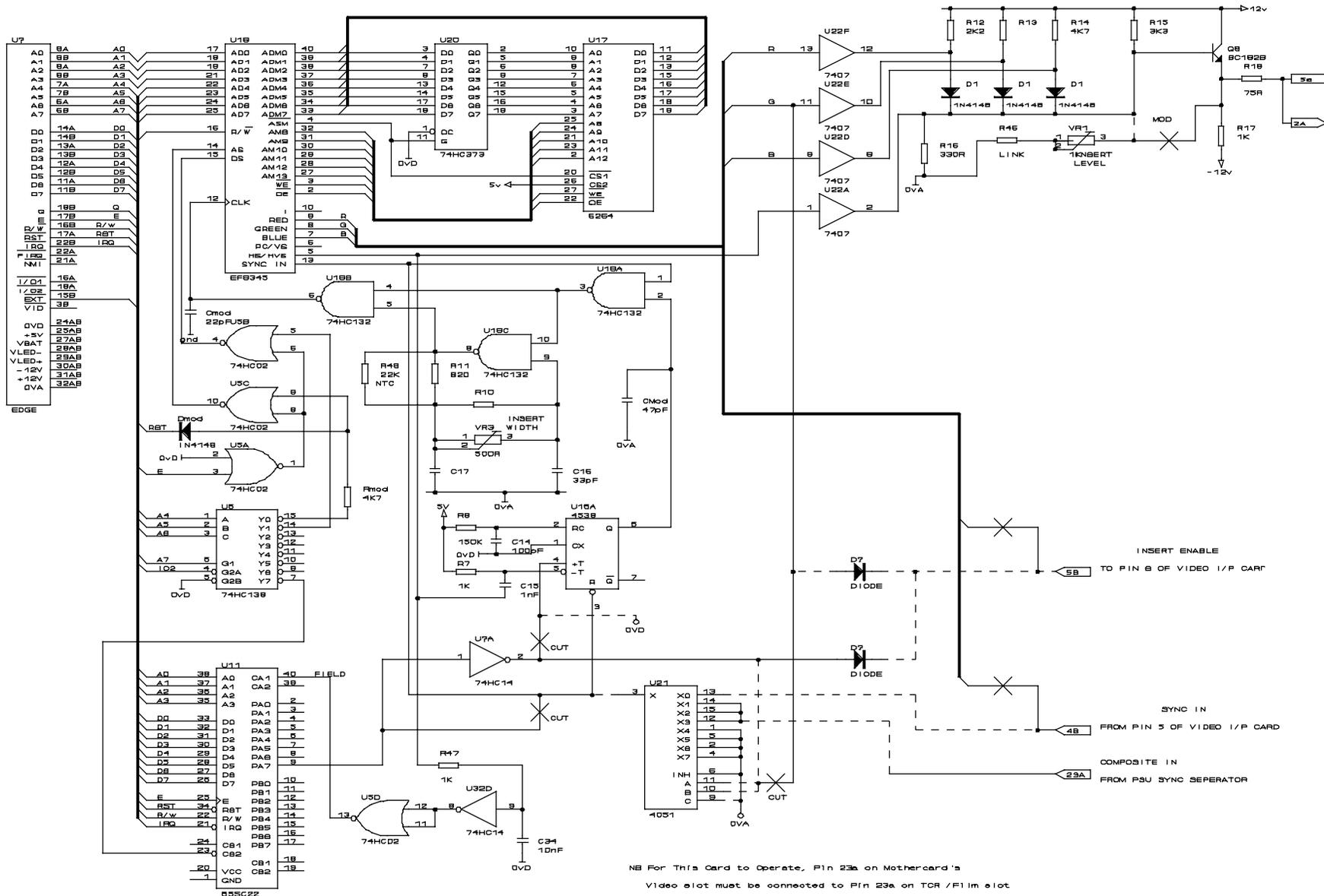
NB For This Card to Operate, Pin 23a on Mothercard's Video slot must be connected to Pin 29a on TCR /Flim slot and U3 pin 1 should be connected to 29a on PSU card. Also cut track leading to pin 29a on TCR card.
