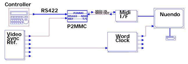
Using the P2MMC with Nuendo as a Device as part of a multiple machine system.
