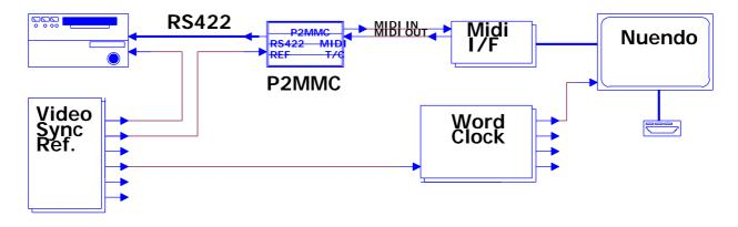
Using the P2MMC with SR-424 to provide multiple machine control from Nuendo.
